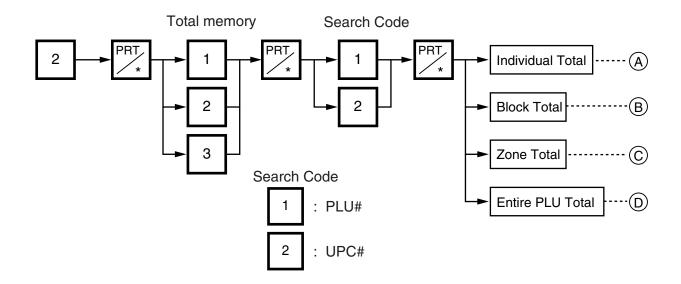
(A) Individual Total Ex.) Individual PLU Total (PLU #100) 0 0 1 (B) Block Total Ex.) UPC Block Total (UPC #100100~100199) 0 0 1  $\diamond$  $\diamond$ **NOTE:** The  $| \diamondsuit |$  key represents 0 through 9. The most significant digit in the starting number is followed by an appropriate number of  $|\diamondsuit|$  keys. (C) Zone Total Ex.) PLU Zone Total (PLU #100~107) 0 0 0 1 1 7 FOR (D) Entire PLU Total
